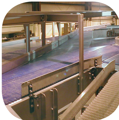
This system was designed to single file shrink wrapped bundles of ice cream in a 0°F operating temperature. It features a drop-out take away conveyor for misoriented bundles.
