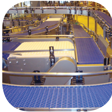
This secondary packaging line utilizes Acetal chain for reduced maintenance in cold environments.
