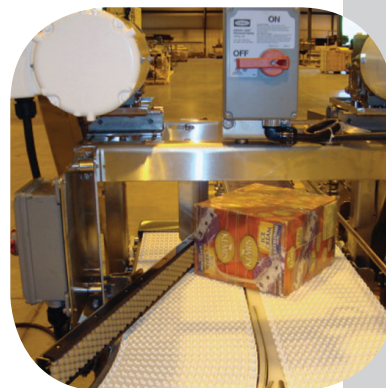
Plastic belt systems provide ease of layout in this six-pack ice cream bundle handling application.
