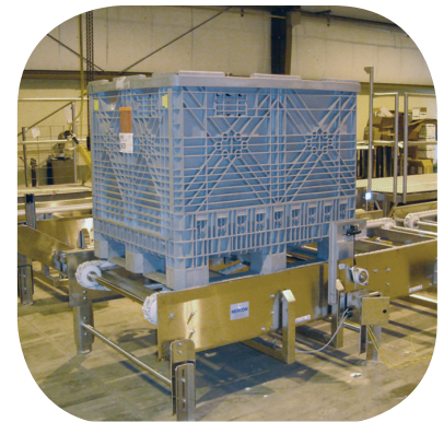
Specially engineered for a 35°F environment, this stainless steel, dual strand, pallet handling system was fully automated and designed to replace manual operations.
