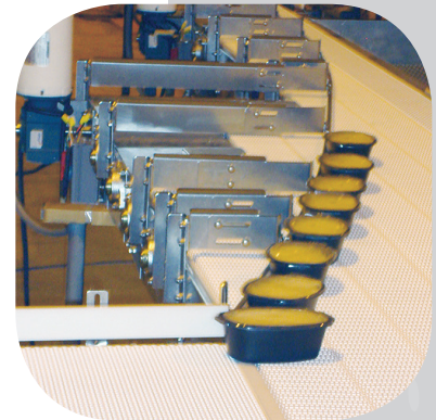
This pressureless single filer effectively aligns frozen food trays along the long axis of the package.
