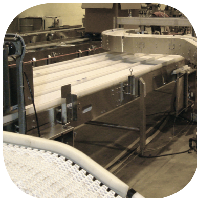
This mat-style system features multiple spurs using overhead servo merges to combine form-and-fill packages of frozen appetizers.
