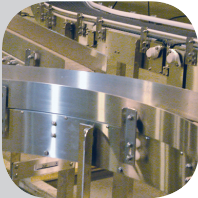
The Sanitary Level I conveyors handle primary packaged food products such as ice cream and other dairy products. This bolted construction design features food grade bearings and sanitary motors/reducers and will handle high pressure, corrosive wash down procedures.
