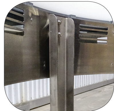
The Sanitary Level III defined as the same environment as Sanitary Level II, is an open frame design, highly polished stainless steel material to facilitate removal of bacteria and biofilms.
