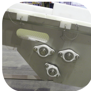
This sanitary incline conveyor shows clean-out holes and removable guide rails.
