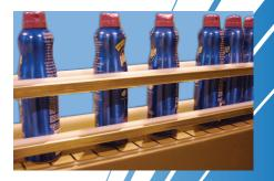
**Tabletop Chain Conveyors** Tabletop chain conveyors are a single product flow accumulation solution. The accumulation occurs in the gaps between the products.
