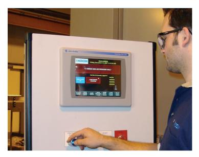
Adding to the efficiency of the packaging line, a HMI (Human Machine Interface) panel allows for programming and automation of different recipes and package sizes, as well as machine and line monitoring.
