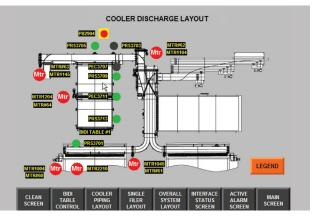
HMI (Human Machine Interface) operator screen showing a multiple cooler discharge system utilizing bi-directional accumulation tables.
