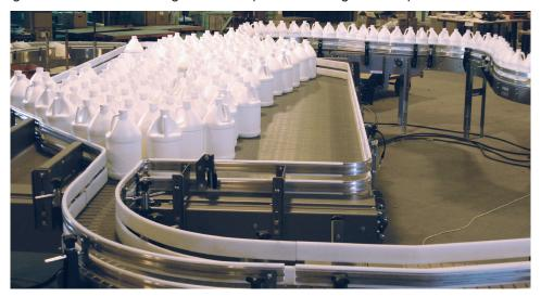
Re-Flow Accumulation Table showing In-Line Accumulation
