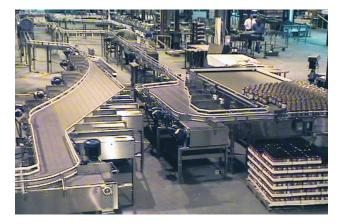
This system uses expanded and optimized electrical controls to integrate all thermal controls and the processes in the high speed sauce line. The line was fully automated an menu driven with multiple HMI's.
