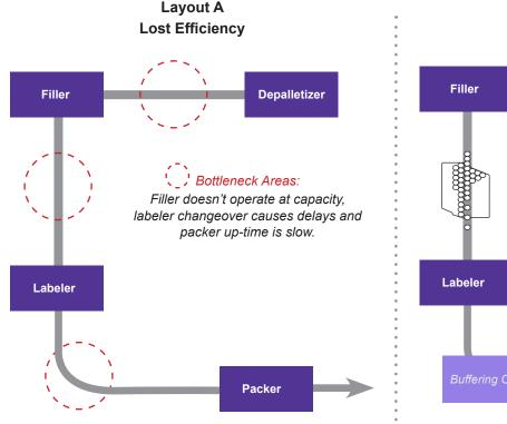
Layout A illustrates four machines in a production line, each operating at 90% efficiency. Whether planned or unplanned, the machines in this example almost never shut down at the same time, resulting in a loss of 40% efficiency.
