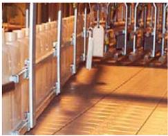
Depending on the type of products and speeds, powered side rails can be a stand-alone merge solution or it is often an added device to assist products as they come in contact with the rail.
