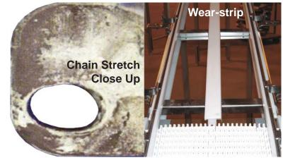
**Chain Stretch:** Over time, the pin housings stretch from a round to an oval shape causing the entire chain length to grow. **Wear-strip:** A wear-strip is the supported guide of the chain and is also a consideration of the application. Wear-strips can be made of plastic, wood, steel or brass.
