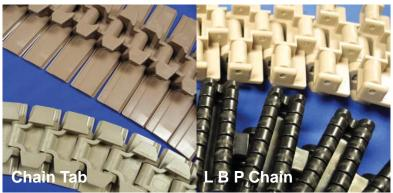
**Chain Tab:** Under Tabletop chain, tabs guide and drive the chain.
