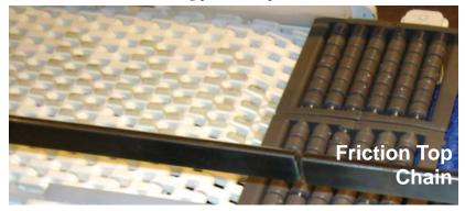
This conveyor was used to transport tissue cartons to a high speed divert system (440 fpm). The high speed pusher required package spacing to direct individual packages into different lanes. The rubber top UNI (PP-PA66-SNB-M2-20) chain maintained the stability of package spacing while being controlled at high speeds.
