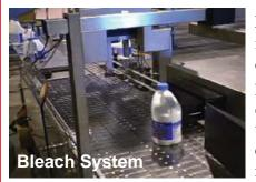
**Chemical:** Production lines where products have chemical spillage or when chemicals are used in the cleaning process are both examples of a chemical environment. For constant chemical exposure, stainless steel chain and pins are preferred. The MSDS provides chemical breakdowns which can be used in consultation with the chain manufacturer for proper chain material selection.
