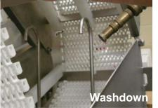
Acetal chains. Polypropylene material, however, will be able to withstand a wash-down environment. The pin material in the chain must also be a consideration. In a wet environment, nylon pins absorb water, causing functional problems and overall weakening of the pins. The MSDS (Material Safety Data Sheet) provides chemical breakdowns of cleaning compounds which can then be compared to the chain manufacturer's material recommendations.
