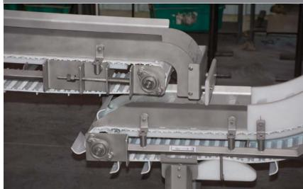
This sanitary freezer room system was engineered for handling bulk frozen food in a -20°F manufacturing environment. The chain used was Intralox Series 800, made from Acetal material with polyethylene pins.
