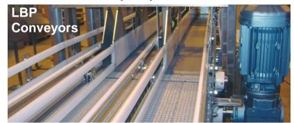
The application called for 30 feet of conveyor feeding case packing operations. The product was a liquid filled PET bottle, labeled and shrink wrapped into 4-pack bundles. Rexnord's LBP821 provided low back pressure during accumulation for short case packer down-times. The chain reduces motor requirements and product damage.
