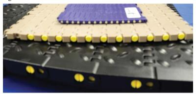
**Pitch:** Pitch is the measurement between pins. The black chain above has a large pitch that might be used for handling cartons or cases. The blue chain above that has a small pitch is used for a noser conveyor.
