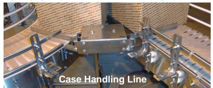
On this slow to moderate speed case handling line; the conveyor shown on the right uses Rexnord LF882, a side flexing chain with low friction properties needed during case accumulation. The chain in the left is Rexnord LF1873 with similar side flexing and low-friction properties, but allows for greater loads needed on that line.
