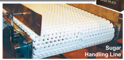
Handling bags of sugar, this chain was an open-grid architecture so sugar could drop out of the conveyor when bags were damaged or leaking. The Habasit chain M3840 was made from abrasion resistant material, including pins and sprockets.
