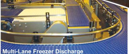
In this three lane freezer discharge conveyor application, Intralox series 2400 matstyle chain was specified. The acetal chain, rated for freezer room temperatures, operates in a -20°F room. The 12" wide, side flexing chain carries bundles of ice cream to down-stream operations. Nylon pins were specified for this application.
