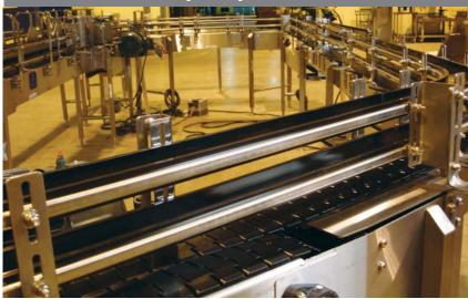
This system was designed for various types of hair care products. The flammable nature of the hair products and the aerosol packaging created the demand for an anti-static system. The Rexnord AS880TAB-K 3-1/4" tabletop chain was used, as well as antistatic guide rails, wear strips and explosion proof motors.
