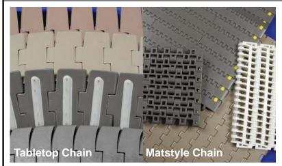
**Tabletop Chains:** Are popular for package and product handling. Common widths start at 3 1/4" through 12". **Plastic Matstyle Chains:** Come in a wide variety of closed or open designs and their construction allows application flexibility.
