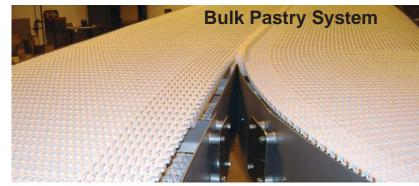
This system was engineered to convey small, bulk pastries at 50 FPM (feet per minute.) A small pitch was required around nosers and limited floor space demanded tight side flexing chain. Rexnord chain WSM1285 was specified for the application. The 30" wide, white chain was sanitation friendly.
