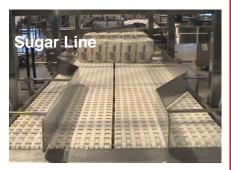
Abrasive: Whether caused by the product running on the conveyor, or a condition of the plant, abrasive environments also require special chain consideration. Cardboard build-up, broken glass, baking flours, cocoa powder and cereals are also examples of abrasive materials. This matter will wear away any chain material, but stainless steel sprockets and abrasion resistant rods will help to increase belt life.
