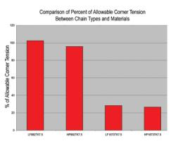
This chart, courtesy of Rexnord Industries, compares two types of chain materials, a low friction series (LF) and a high performance (HP) series. In this comparison example, both HP series chains have less horse power requirements than the low-friction chain. It is interesting to note that the material in HP chain has high slip properties; greater than the LF material.
