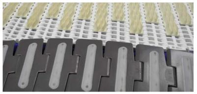
**Friction Chain:** Friction inserts are available on both tabletop and matstyle chains - used to prevent product slipping.
