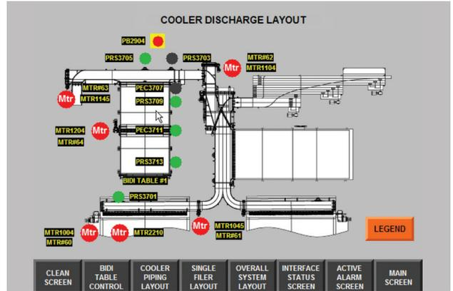
HMI (Human Machine Interface) operator screen showing a multiple cooler discharge system utilizing bi-directional accumulation tables.
