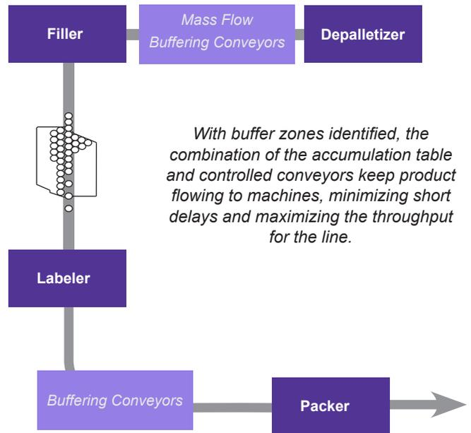
Layout B shows the same four machine scenario with accumulation and buffering planned into the line, resulting in reclaiming the lost efficiency.
