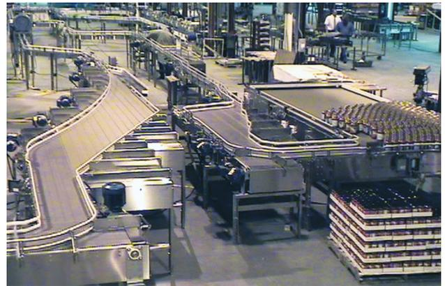
This system uses expanded and optimized electrical controls to integrate all thermal controls and the processes in the high speed sauce line. The line was fully automated an menu driven with multiple HMI's.
